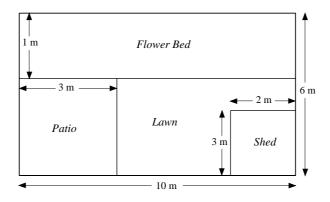
Produce a scale drawing with a scale of 1: 200.
