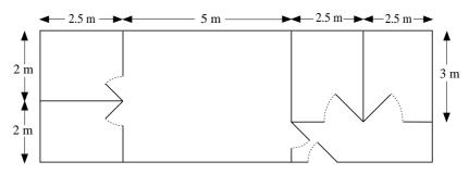
Use the information given to produce a scale drawing with a scale of 1: 200.
